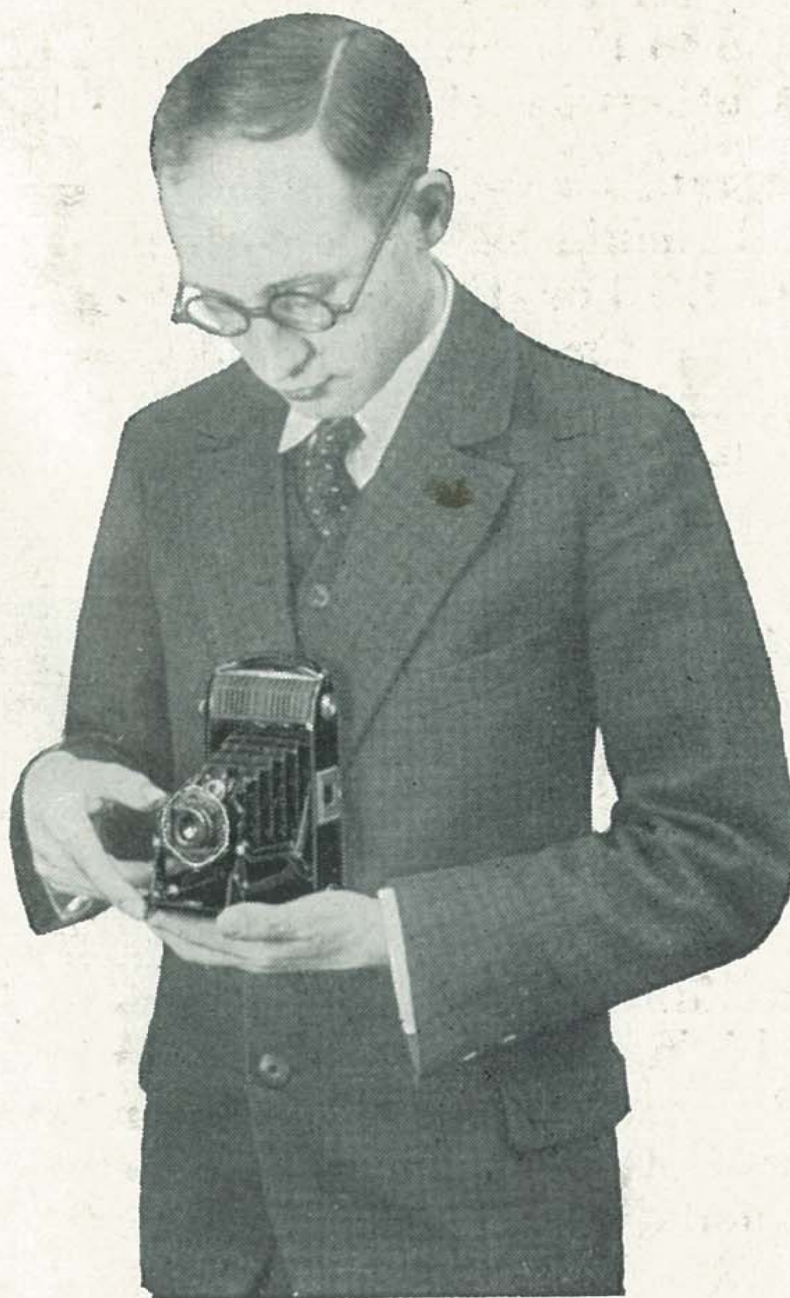
Fig. 4 How to hold the camera for a vertical exposure, when using the brilliant view finder
